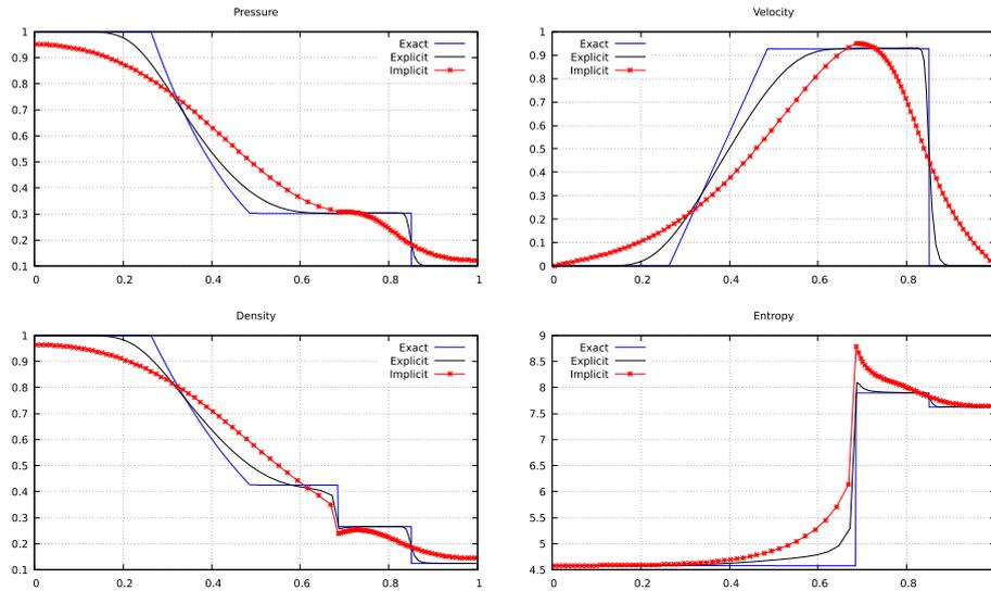
FIGURE 2. Sod shock tube for Euler equations. The CFL are  $CFL_{\text{explicit}} = 40$  and  $CFL_{\text{implicit}} = 40$ .
