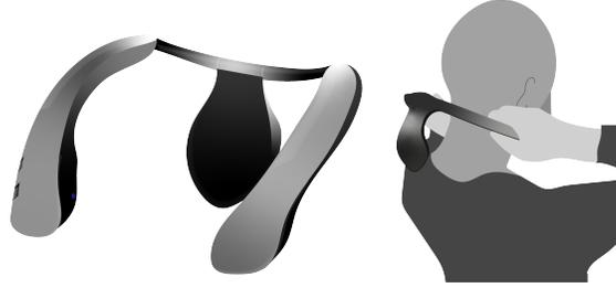
**Fig. 3.** The product design artifact. A preliminary illustration of the future Ryzm™ device, designed for tactile augmentation of listening. The device integrates three positions of vibrotactile stimulation on the upper neck and clavicles.
