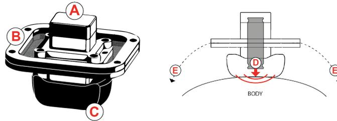
**Fig. 2.** The vibratory module. The module snaps onto extended fabric, tightened between the edges of the frame (B). A rounded, hard bottom (C) comes into contact with the body, transmitting the vibrations of the actuator to the user. The actuator’s axis of vibration (D) is orthogonal to the body’s surface. It “breathes” within its structural frame, and is pulled against the body by straps attached at all four corners (E).
