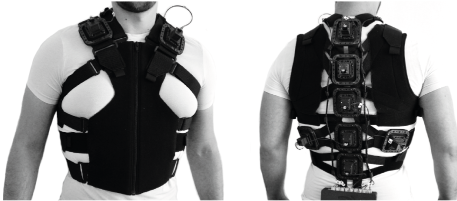
Fig. 1. The multimodal harness. Nine voice-coil motors (Actronika HapCoil) are integrated in the wearable structure inside hard plastic modules on the clavicles, spine and ribs. The velcro straps tighten the modules' contact against the body, whose vibrations penetrate the body to elicit ETC sound perception, and stimulate the skin for tactile sensations. Users receive earplugs and a noise-reducing headset (3M Peltor X5A) in order to protect them from all external noises created by the actuators and ensure they hear only via ETC.
