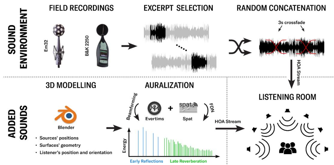
Figure 2: Flowchart of the soundscape simulation tool. The ambient **sound environment** (upper part) is simulated from concatenated excerpts from fields HOA recordings. A 3D Modelling of the scene is sent to an auralization unit that converts monophonic **added sounds** (lower part) to HOA streams. Both streams are diffused in a listening room for soundscape evaluation.
