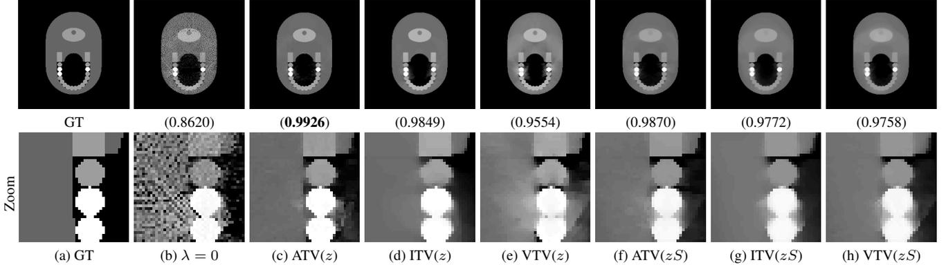
**Fig. 3: Comparison of different regularization strategies for the proposed method.** The first row shows the average attenuation coefficients reconstruction for different settings, along with the SSIM score in parenthesis. The second row shows a close-up view of a dental area where metal implants are present.
