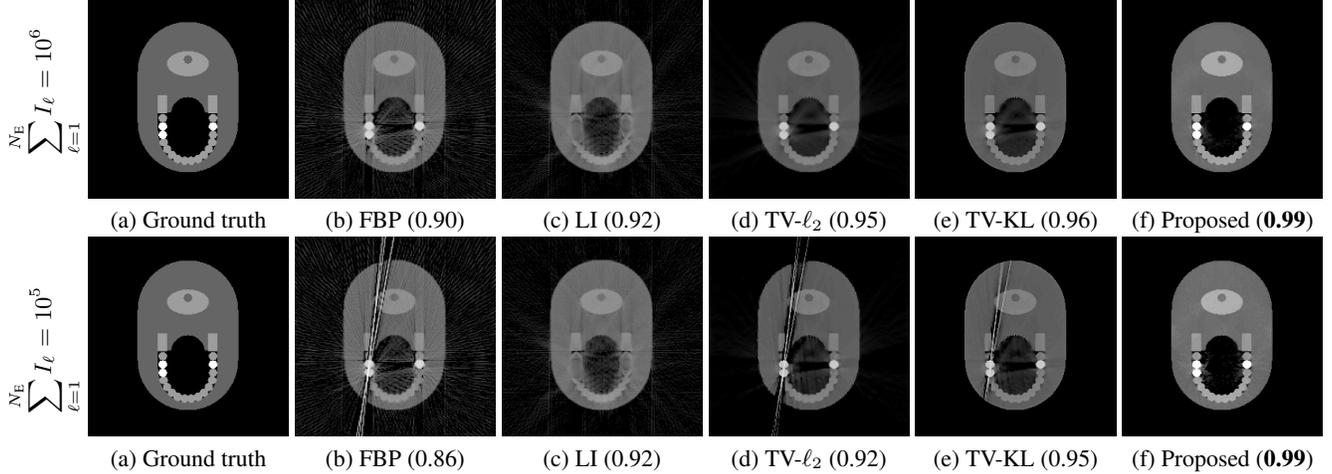
**Fig. 2: Comparison of beam hardening artifacts reduction methods in CT, in normal (first row) or low (second row) photon counts, with the same notations as in Fig. 1 (displaying the reconstructed average attenuation coefficients  $\bar{\mu}$ ). Low photon counts further amplify metal artifacts in existing CT reconstruction techniques, while the proposed one remains robust even in this challenging setting.**
