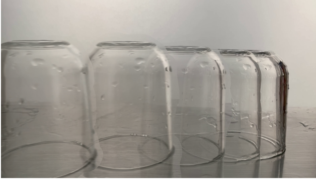
FIG. 1. Warm glass moving spontaneously from right to left after being put on a glass surface. The surface initially coated with a thin layer of soap water and was intentionally tilted by \simeq 1 degree to drive the motion. The width of the field of view is \simeq 50 cm and the time between shots is \simeq 0.5 s
