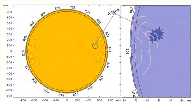
**Figure 8:** The left image depicts a 2D plot of a lateral section of the breast, as for the right one it is the way the acoustic wave is diffracted from the emitter to the receiver.
