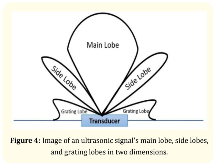
**Figure 4:** Image of an ultrasonic signal's main lobe, side lobes, and grating lobes in two dimensions.
