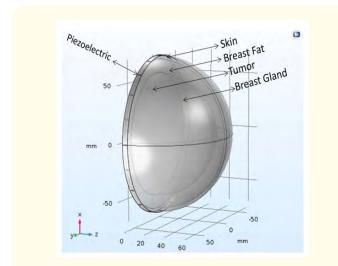
Figure 5: FEM 3D model of the female breast with tumor.
