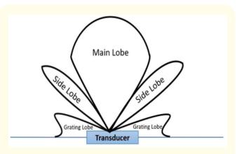
Figure 4: Image of an ultrasonic signal's main lobe, side lobes, and grating lobes in two dimensions.
