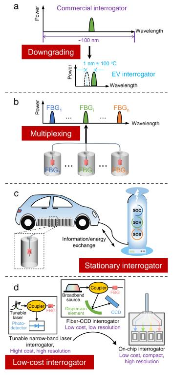
**Figure 3 | Reducing the cost of interrogation. a,** Downgrading the wavelength range of interrogator. **b,** Wavelength division multiplexing of multiple optical sensors in a single interrogation channel. **c,** Stationary interrogator for sharing the interrogation cost. **d,** Low-cost interrogators by fiber-CCD interrogator<sup>36</sup> and on-chip interrogator<sup>37</sup>.
