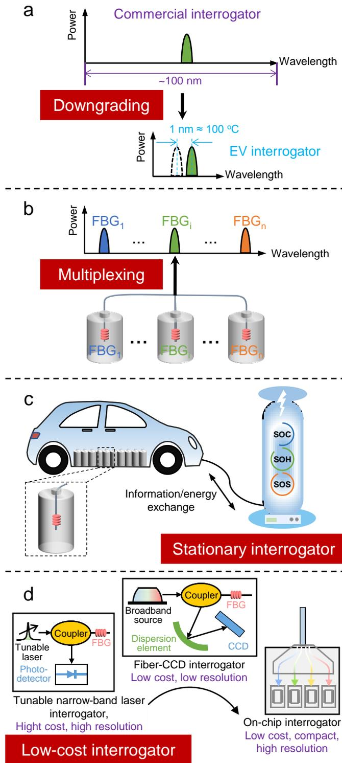
**Figure 3 | Reducing the cost of interrogation.** a, Downgrading the wavelength range of interrogator. b, Wavelength division multiplexing of multiple optical sensors in a single interrogation channel. c, Stationary interrogator for sharing the interrogation cost. d, Low-cost interrogators by fiber-CCD interrogator<sup>36</sup> and on-chip interrogator<sup>37</sup>.
