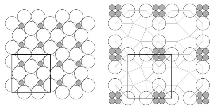
FIG. 5. Reference periodic phases. Black squares highlight the unit cells. (Left) The sigma phase, first approximant of the dodecagonal tiling. (Right) A reference periodic structure based on the large square-small square-isosceles triangle tiling. The octagons can host cluster of variable composition and orientation. Possible fillings are suggested in grey.
