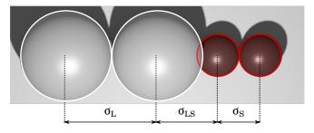
Fig. 1 Schematic depiction of the model. 3D hard spheres lying on a flat surface (top) can be interpreted as an equivalent 2D system of non-additive hard disks (bottom). Spheres of the same type behave like standard hard disks (their projections cannot overlap), while the closest projected distance between particles of different types  $\sigma_{LS}$  is smaller than the sum of the radii.
