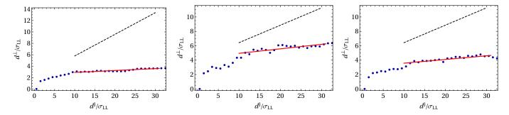
Fig. 6 The average perpendicular displacement  $d^{\perp}$  as a function of the parallel-space displacement  $d^{\parallel}$  for the three self-assembled quasicrystal configurations in Fig. 4. The red lines are linear fits to the large-distance behavior, with the slope related to the average perpendicular strain. For comparison, we also plot the corresponding line for a periodic approximant for each system (dotted black lines).
