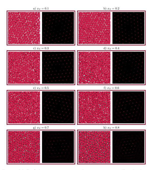
FIG. 1. Variations of the  $\text{Hex}_{\text{L}}^+$  phase, at size ratio q = 0.35 and varying compositions  $x_S$ . The packing fractions for the snapshots vary from  $\eta = 0.82$  in (a) to  $\eta = 0.96$  in (h), in steps of 0.02.
