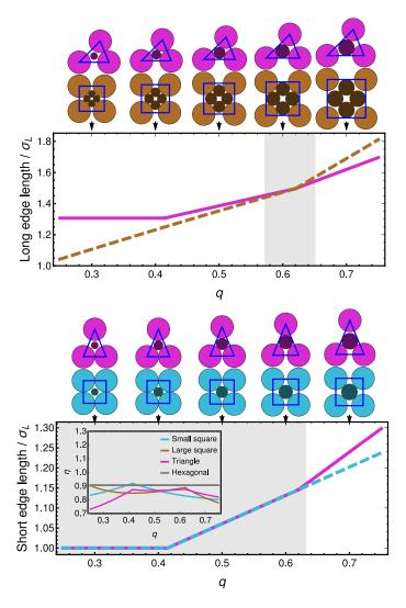
FIG. 6. Comparison of the long (top) and short (bottom) edge length of the tiles expected to form an octagonal quasicrystal in binary mixtures of *additive* hard disks. Size ratio intervals for which long or short edges match are highlighted with a darker background. The inset in the bottom graph displays the packing fraction of the various tiles as a function of size ratio, along with that of hexagonal packings.
