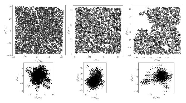
FIG. 4. Parallel (Top) and perpendicular (Bottom) projections of the lifted tilings. (Left) QC12 q=0.45,  $x_S=0.35$ ,  $\eta=0.84$ . (Centre) QC8 q=0.5,  $x_S=0.675$ ,  $\eta=0.86$ . (Right) QC8 q=0.55,  $x_S=0.725$ ,  $\eta=0.84$ . The empty region in to top right corner corresponds to a fluid pocket with no tiling structure.
