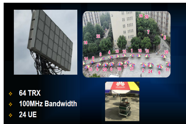
Fig. 2. The 5G base-station prototype
