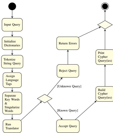
Fig. 1. Activity Diagram. Shows program processing steps.
