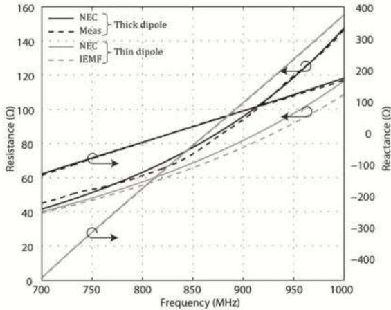
Figure 2: Input impedance of an isolated thin and thick dipole.
