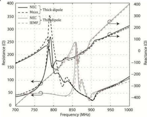
Figure 3: Input impedance of dipole no.1 in  $\lambda \times \lambda$  distribution area.
