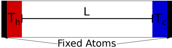
Fig. 2. Schematic representation of a NEMD simulation set-up with the hot region in red and the cold region in blue at the two extremities of the structure. To avoid distortion of the nanostructure some layers of fixed atoms are usually used after the thermostats. The extraction of the thermal properties concerns the distance L as depicted in the figure.
