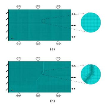
FIG. 3. (Color online) Illustration of mesh of the P-S conversion model by XFEM (a) and FEM (b).
