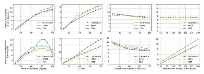
FIG. 7. (Color online) Results of the parametric study presenting the variation of angle of refraction  $\alpha_t$  and amplitude  $A_t$  of transmitted S-waves across an oblique linear interface, in terms of the parameters, including angle of incidence  $\alpha_i$ , modulus  $E_{\infty}$  of material 2, frequency f, and amplitude  $A_i$  of incident P-waves.
