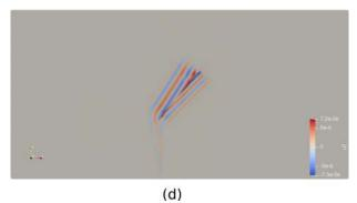
FIG. 6. (Color online) Illustration of displacement fields and extracted Swaves of the P-S conversion model with the default parameters. (a) and (b), from the model by XFEM, present the displacement fields along *x*-axis and *y*-axis, respectively. (c) and (d) present the extracted S-waves from the displacements of model by XFEM and FEM, respectively.
