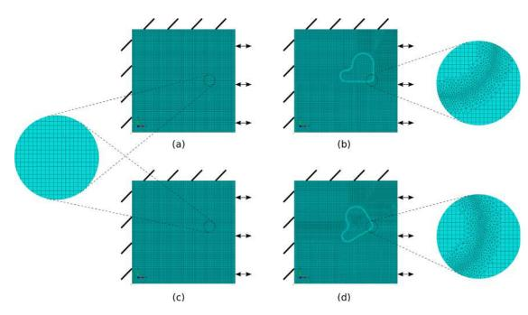
FIG. 5. (Color online) Illustration of mesh of the random-shape inclusion model by XFEM and FEM. (a) and (c) present the regular mesh by XFEM for the *aligned* and *tilted* inclusion, respectively. (b) and (d) present the mesh by FEM for the *aligned* and *tilted* inclusion, respectively, where triangular elements are used to match the material interface.
