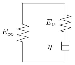
FIG. 1. Maxwell form of SLS model.
