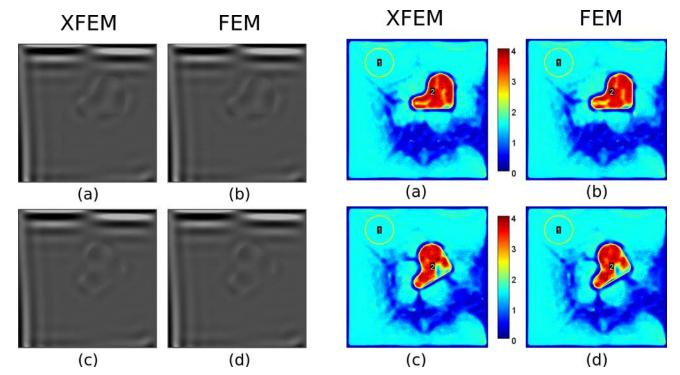
FIG. 8. Illustration of the first snapshot during a period in steady state (100th period) of curl-applied displacement fields  $u_T$  from the model containing a random-shape inclusion. (a) and (c) correspond to the results of XFEM simulation for the *aligned* and *tilted* inclusion, respectively, while (b) and (d) correspond to the results of FEM simulation for the *aligned* and *tilted* inclusion, respectively.
