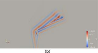
FIG. 10. (Color online) Illustration of converted S-waves by the P-S conversion XFEM model with the angle of incidence  $\alpha_i = 60$  degrees. A central zoom is taken for illustration purpose. (a) corresponds to the model meshed with element size of 2 mm, while (b) corresponds to the model with element size of 1 mm.
