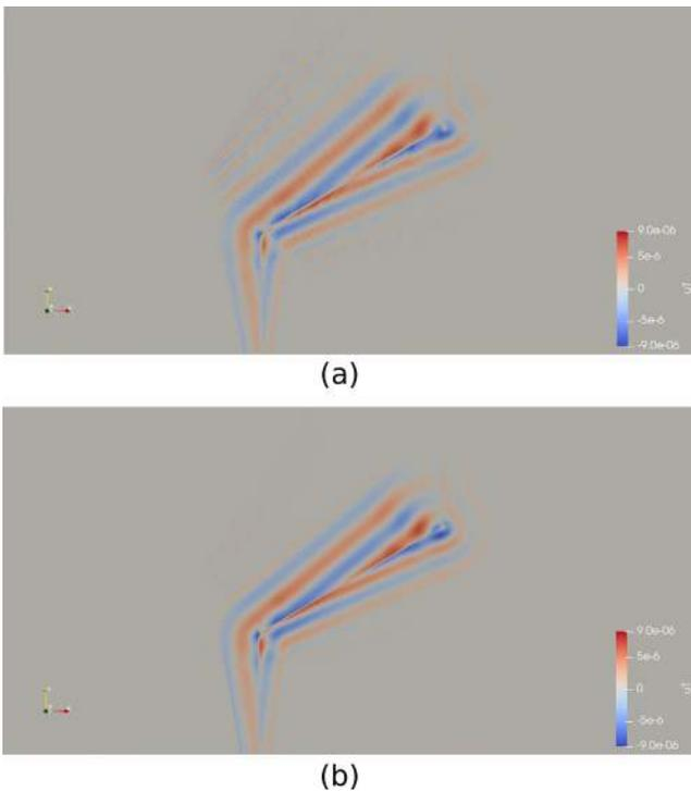
FIG. 10. (Color online) Illustration of converted S-waves by the P-S conversion XFEM model with the angle of incidence  $\alpha_i = 60$  degrees. A central zoom is taken for illustration purpose. (a) corresponds to the model meshed with element size of 2 mm, while (b) corresponds to the model with element size of 1 mm.
