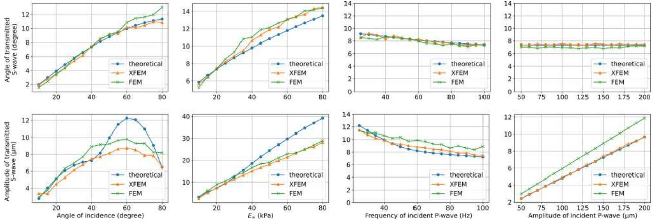
FIG. 7. (Color online) Results of the parametric study presenting the variation of angle of refraction  $\alpha_t$  and amplitude  $A_t$  of transmitted S-waves across an oblique linear interface, in terms of the parameters, including angle of incidence  $\alpha_i$ , modulus  $E_\infty$  of material 2, frequency  $f$ , and amplitude  $A_i$  of incident P-waves.
