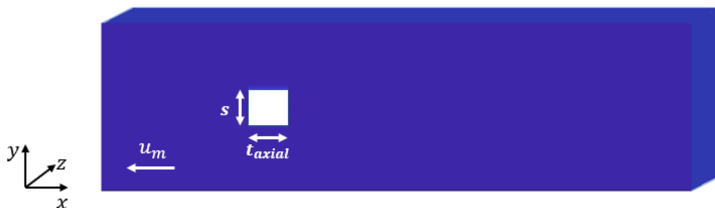
Figure 2: Liner surface with a moving heat flux
