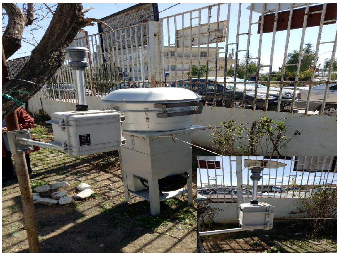
Fig. S2. Sampler (LVS) used for sampling aerosols at the Zouaghi site
