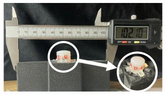
(a) A stimulus (Shore 00-10 R=21.4 mm) installed on 3D-printed support for the curvature measurement. A vernier scale is fixed on the support to make sure the precision of conversion of our measurement on pixels to mm.
