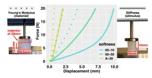
(a) Compression tests: Young's Modulus (dotted line, left) measured following the standard [23]. The indentor is 3D printed with rigid resin; The stiffness (solid line, right) measured with specimens with the same dimension as the stimuli used in our experiment.
