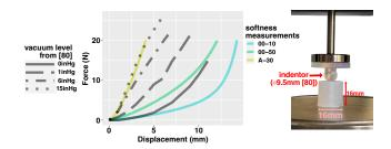
Figure 10: (Left) Force displacement curves resulting from (right) compression tests with a 3D printed spherical indentor as in [80]. Colored lines show our results on a specimen with the same dimensions as the stimuli used in our experiment. Gray lines show prior results [80] from compression test on a jamming layer. The level of vacuum are expressed in inches of mercury (inHg). The larger the value, the higher the vacuum and the stiffer the UI.
