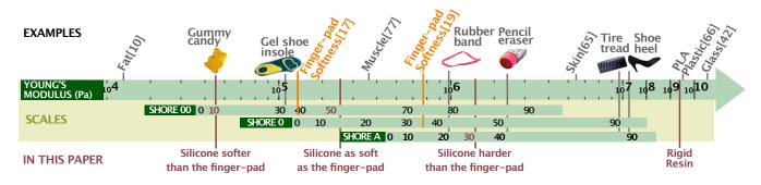
Figure 1: (Top) Example materials and objects and (center) their approximate Young's modulus [21] and respective Shore hardness [22]. (Bottom) Types of silicone and resin used in our experiment: Shore 00-10, Shore 00-50, Shore A-30, and Rigid.
