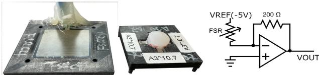
(d) (Left) The pressure sensor Interlink FSR406 stuck on the 3D printed support and (middle) a stimulus to install on this support. (Right) The schematics of the circuit for sensor reading (as in [27]).
