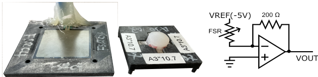
(d) (Left) The pressure sensor Interlink FSR406 stuck on the 3D printed support and (middle) a stimulus to install on this support. (Right) The schematics of the circuit for sensor reading (as in [27]).
