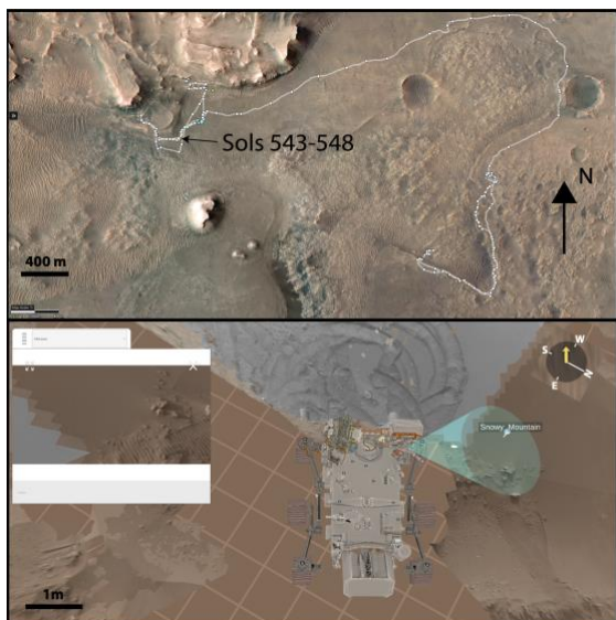
Figure 2. (Top) HiRISE map showing the trajectory of Perseverance during the first 667 sols of the mission. The blue and green dots indicate the position of the rover and Ingenuity on sol 667. (Bottom) Field of view of the ground temperature sensor (shaded green area) on sols 543-548, which included the SuperCam target called Snowy Mountain. A zoomed-in view of the field of view is shown on the top left insert.
