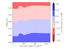
Fig. 5: Stability of the robot along  $\mathcal{P}$  versus the position estimation error  $\delta^w \mathbf{t}_p$
