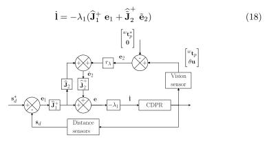
Fig. 3: Control scheme of the CDPR with the fusion of the distance and pose errors.
