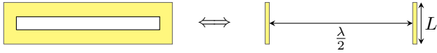
Fig. 4. Equivalent model of the loop resonator. The loop is replaced by two small dipoles spaced \lambda/2 apart with \lambda taken at the fundamental resonance frequency of the loop f_1 .
