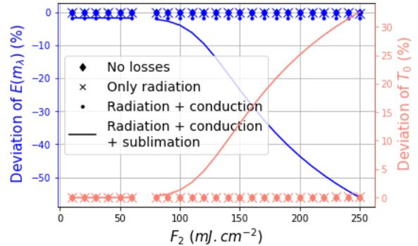
Figure 3: Deviations of  $E(m_\lambda)$  (blue line) and of  $T_0$  (pink line) from their reference values, as a function of  $F_2$  when different loss terms are considered in Eq. (1): no losses ( $\diamond$ ), radiation ( $\times$ ), radiation and conduction ( $\bullet$ ), and radiation, conduction and sublimation (solid lines).
