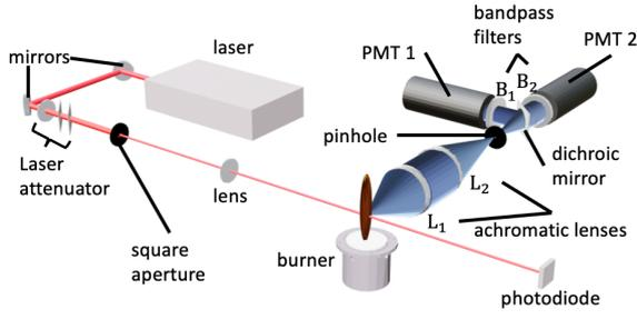
Figure 2: Scheme of the LII experimental bench.
