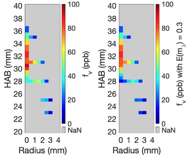
Figure 8: Left: distribution of  $f_v$ , computed using the spatial evolution of  $E(m_\lambda)$  of Fig. 7. Right: distribution of  $f_v$  computed considering a spatially uniform  $E(m_\lambda) = 0.3$ .
