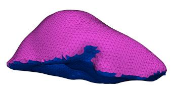
(a) Initial mesh. The bottom surface (in blue) is the loaded surface while the top surface (in magenta) is the matching surface.
