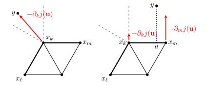
Figure 2: Illustration of  $\nabla j(\mathbf{u})$  in two configurations. Points  $x_{\ell}$ ,  $x_k$  and  $x_m$  are located on the mesh boundary, while the last vertex is inside the mesh. The red arrows represent the components of the descent direction  $-\nabla j(\mathbf{u})$ . On the right, the equality  $y - a = -\partial_k j(\mathbf{u}) - \partial_m j(\mathbf{u})$  holds.
