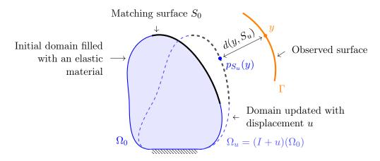
Figure 1: Problem geometry. The thick dashed line represents the deformed matching surface  $S_u$ . The distance between a point  $y \in \Gamma$  and its orthogonal projection onto  $S_u$  is denoted by  $d(y, S_u)$ .
