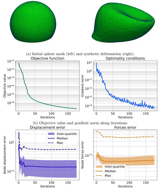
(c) Reconstruction error statistics for vertex displacements and nodal forces.
