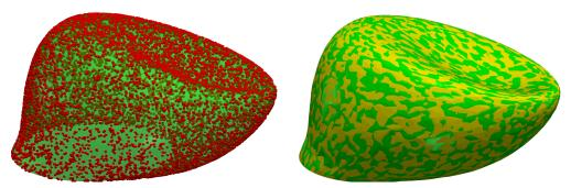
(a) Point cloud and superposition of the true and reconstructed surface.
