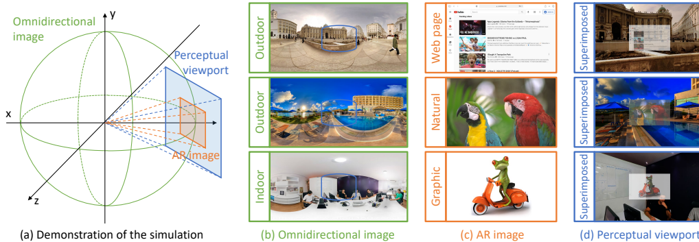
Fig. 12. The illustration of the AR simulation in VR environment. (a) The demonstration of the relationship between the omnidirectional image, the AR image, and the perceptual viewport image. (b) The omnidirectional images are used as the background scenes, which include outdoor and indoor scenarios. (c) The AR images are composed of three types of content including web page images, natural images, and graphic images. (d) The perceptual viewport images are generated by superimposing the AR images on the omnidirectional images (here \lambda = 0.58 ). Note that the perceptual viewpoints of the subjects are changed dynamically with the head movement, however, the relative positional relationship between the omnidirectional image and the AR image is fixed.
