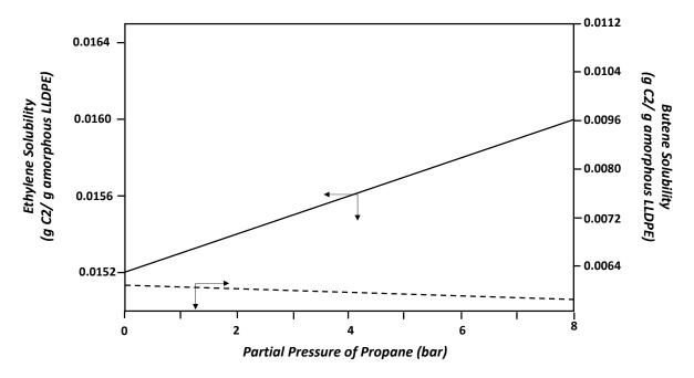
Figure 5. Example of the cosolubility effect of propane on a mixture of 7 bars of ethylene and 1 bar of 1-butene at  $70^{\circ}$ C.
