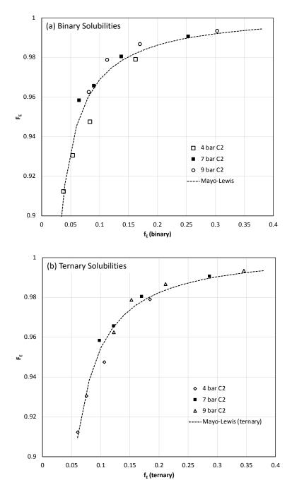
Figure 2. Copolymer composition versus monomer composition in amorphous fraction of the polymer of (a) binary and (b) ternary solubility calculations for ethylene/1-hexene copolymers.
