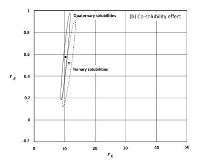
Figure 4. Plot of 95% joint confidence region for ethylene/1-butene copolymerization in the presence of isobutane as ICA for (a) pure component solubility and (b) accounting for the cosolubility effect. 7 bars of ethylene, 1 bar 1-C4, 0 and 3 bars of iC4.
