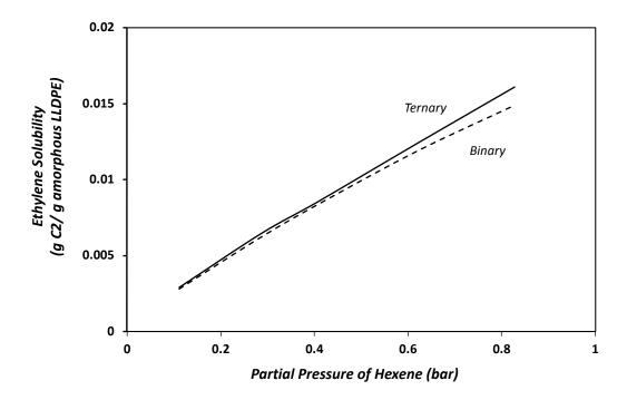
Figure 3. Cosolubility effect of hexene on ethylene (7 bars ethylene, 70°C) represented by the Ternary model. The Binary example does not account for the cosolubility.
