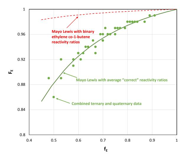
Figure 6. Mayo-Lewis plot for the ensemble of ternary and quaternary data from Tables 6-8 (data points), with an average value of the reactivity ratios estimated using the SL-EOS accounting for interactions (solid line,  $r_E=10.5$ ,  $r_B=0.53$ ) and the copolymer compositions calculated using the binary reactivity ratios in Table7.
