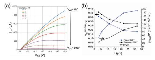
**Figure 2.** a) Typical output  $(I_{DS} - V_{DS})$  curve for a planar PEDOT:PSS-based OECT ( $L = 11 \mu$ m,  $W = 50 \mu$ m). Gate voltages ( $V_{GS}$ ) are biased from 0 V to +0.6 V. b)  $\mu_{OECT}C^*$  product (right) and  $V_{GS}$  at  $g_{m, max}$  (left) as a function of channel length (L) for planar or staggered OECTs.
