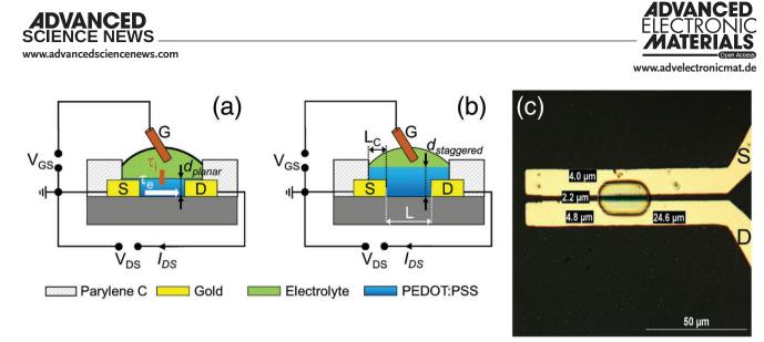
**Figure 1.** Bottom contact—Top Gate (BC-TG) OECT in a) staggered or b) planar architectures. c) Microphotograph of OECT with 45% and 55% channel overlap with S&D electrodes, respectively ( $W \approx 25 \,\mu$ m;  $L = 2.2 \,\mu$ m;  $L_{c^{+}}^{F_{c^{+}}} = 4$  and 4.8  $\mu$ m, respectively). The scale bar is worth 50  $\mu$ m.
