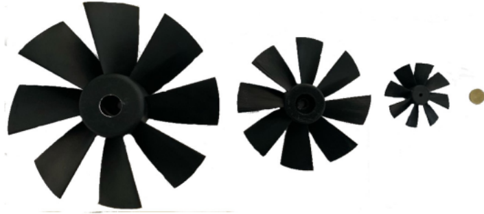
Figure 3: Printed wind turbines used in scaling tests with a 50 euro cent coin
