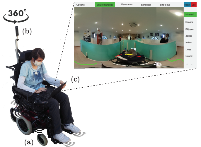
Fig. 1: Overview of system components: (a) Power wheelchair equipped with a ring of range sensors; (b) Twin-fisheye camera; (c) Visualization interface.
