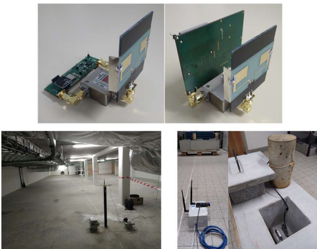
Figure 3. Photographs of: (top) Sensing Nodes, using (right) or not (left) the electronic Printed Circuit Board as a 6 cm x 8 cm metallic reflector plane located 5 cm behind the single antenna; and (bottom) experimental setups of the Cyber-Physical System (left) indoors and (right) with Sensing Nodes embedded in a reinforced concrete beam.
