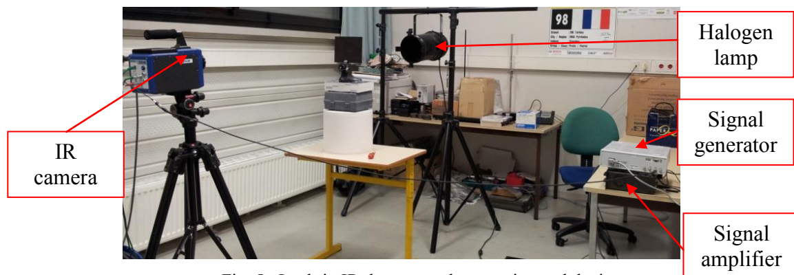
Fig. 5 : Lock-in IR thermography experimental device
