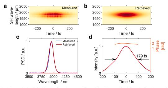
**Fig. 2.** Results of FROG characterization of the solitonic pulse at the output of the InF<sub>3</sub> fiber. (a) Measured and (b) retrieved FROG traces. (c) Spectral profiles retrieved from the FROG trace and measured with the FTIR spectrometer. (d) Retrieved temporal intensity (purple) and phase (orange) profiles. (For interpretation of the references to colour in this figure legend, the reader is referred to the web version of this article.)
