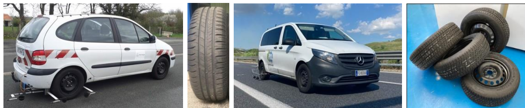
Figure 7. CPX test vehicles and tyres: Renault Scenic fitted with Michelin Energy Saver tyres (left) and Mercedes Vito fitted with SRTT tyres (right)
