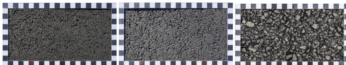
Figure 2. Detailed view of the prototype road surfaces P (left) and PCR (middle), and of the reference road surface E1 (right)
