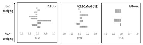
Figure 5 – Evolution of Copper enrichment factors during dredging of Pérols (P), Palavas (PA) and Port-Camargue (PC).
