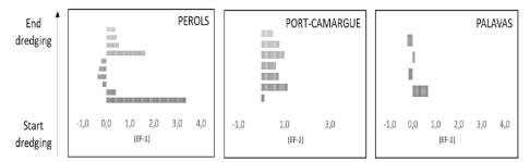
Figure 6 – Evolution of Zinc enrichment factors during dredging of Pérols (P), Palavas (PA) and Port-Camargue (PC).
