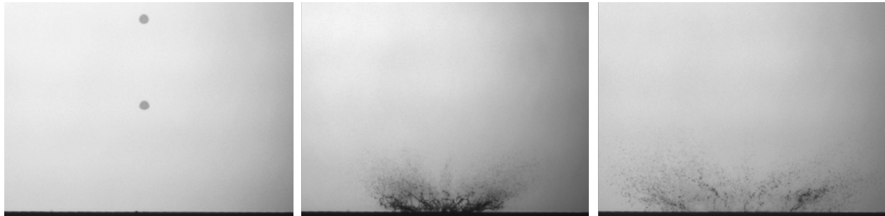
(a) Impact on a dry and smooth surface at 150 m/s.
