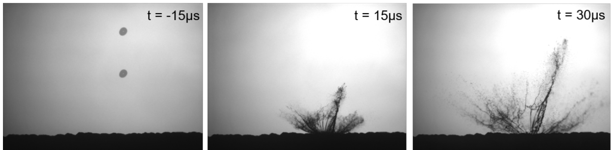
(b) Impact on a glaze ice surface at 150 m/s in an airflow cooled at -2^{\circ}\text{C} .
