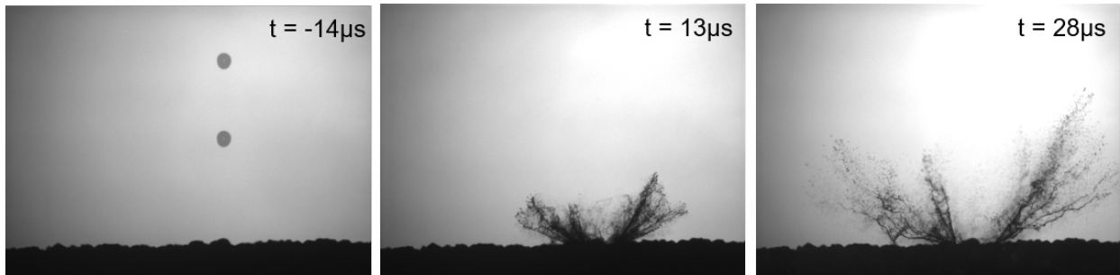
(c) Impact on a rime ice surface at 150 m/s in an airflow cooled at -5^{\circ}\text{C} .
