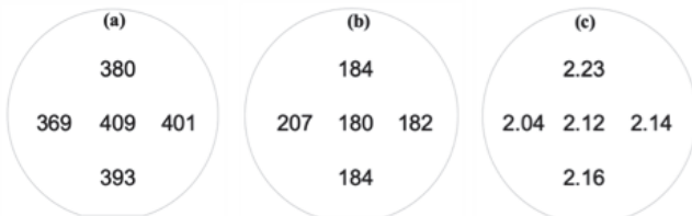
Fig. 7 Electrical properties of the epistructure across the 2-inch epiwafer (a) sheet resistance ( \Omega/\text{sq.} ), (b) mobility ( \text{cm}^2/\text{V.s} ) and (c) carrier density ( \times 10^{18} \text{ cm}^{-3} ).
