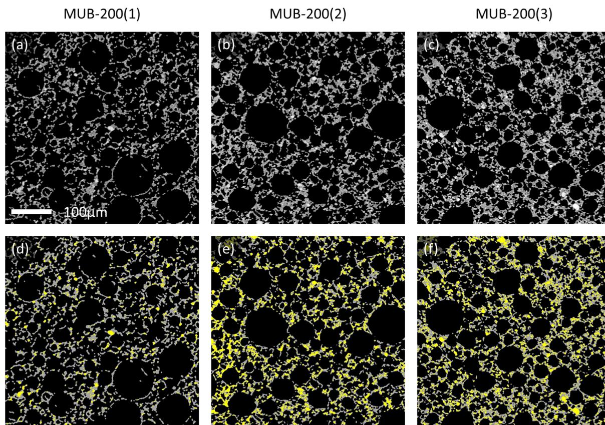
**Figure 3.** (a-c) Digital cut through the 3D X-ray tomographic datasets for the three materials of the MUB-200(x) series. (d-f) false colour image of the same image plane where black represents pores, grey represents the  $\text{SiO}_2$  matrix and yellow the  $\text{TiO}_2$  inclusions.
