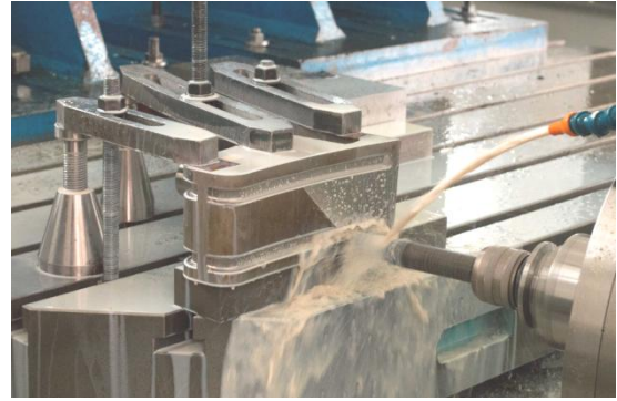
Fig. 5: Drilling of the cooling channels.
