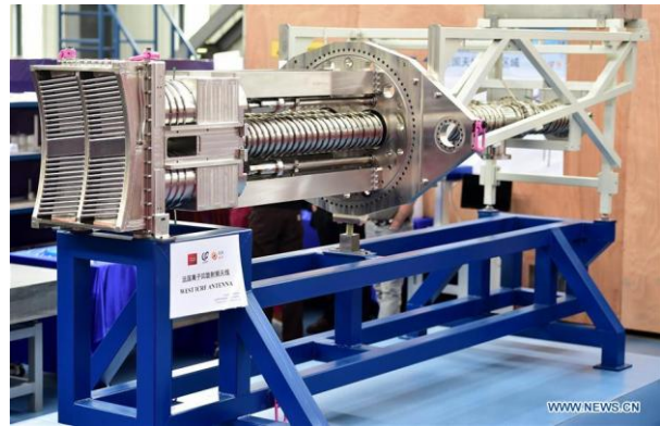
Fig. 9: Antenna blank assembly at ASIPP.
