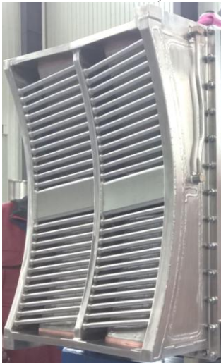
Fig. 8: Finished FS pre-mounted with straps
