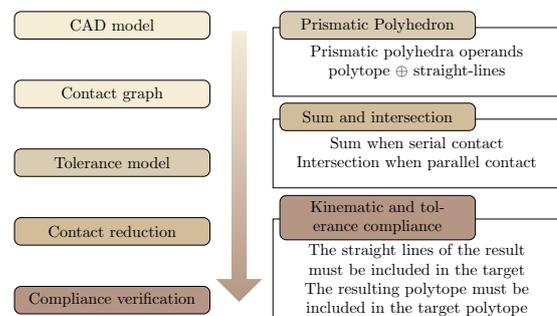
Figure 1: Tolerance analysis with the polyhedral approach
