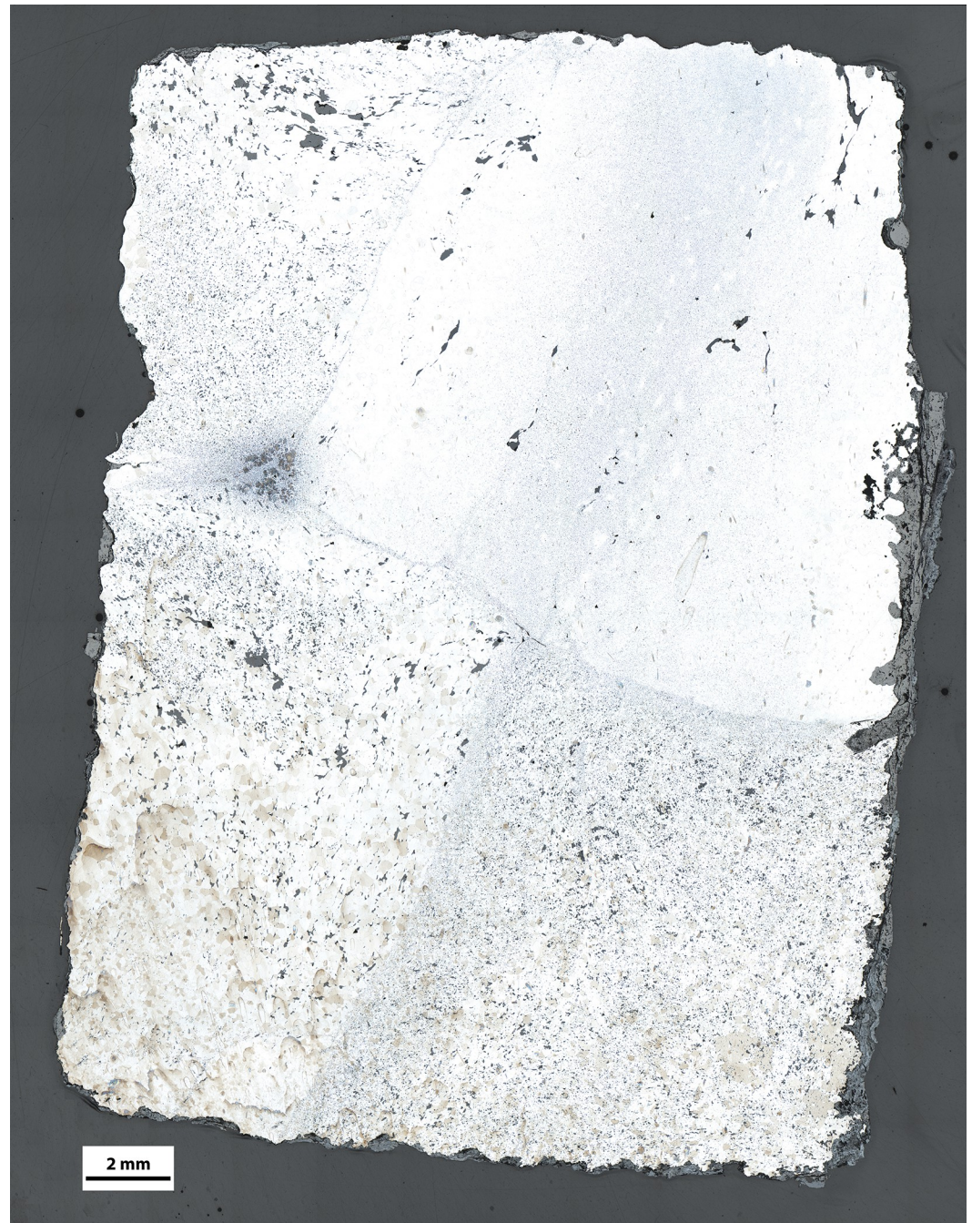
Fig 12. Micrograph of sample VN2-T showing several welding lines and different microstructures (Nital etching).
