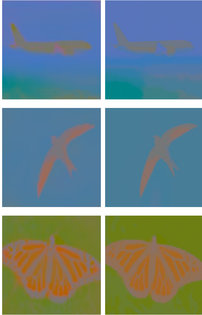
Fig. 7. Chrominance channels. Left: output of CIC [21]. Right: proposed approach (minimization of Eq. (5)). The proposed approach with regularized deep image prior gives a better localization of the chrominance information, which explains reduced color halos. The corresponding color images can be seen in Fig. 2. Best seen on screen.
