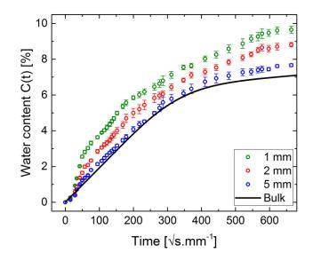
**Figure 6.** Evolution of the macroscopic water content as a function of immersion time for different bonded joint thickness
