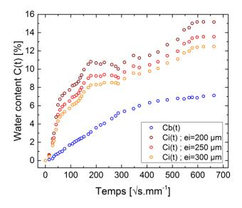
**Figure 10.** Evolution of the water content Cb(t) and Ci(t) as a function of immersion time, calculation carried out using the dual layer model considering three cases for the thickness of the interphase 200, 250 and 300  $\mu$ m.
