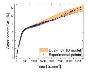
Figure 5. Sorption kinetics of the bulk adhesive during immersion water at 40  $^{\circ}$ C
