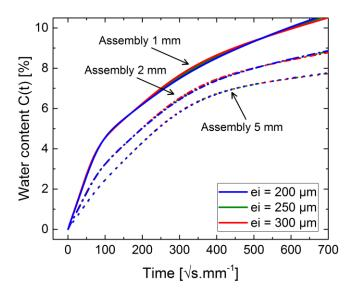
Figure 11. Comparison of the dual layer model on the calculation of the macroscopic water content for three interphase thicknesses: 200, 250 and 300  $\mu$ m
