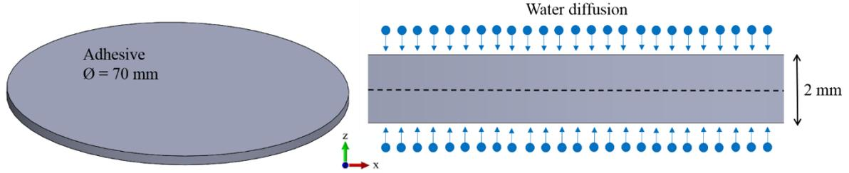
**Fig. 2.** An adhesive disc specimen
