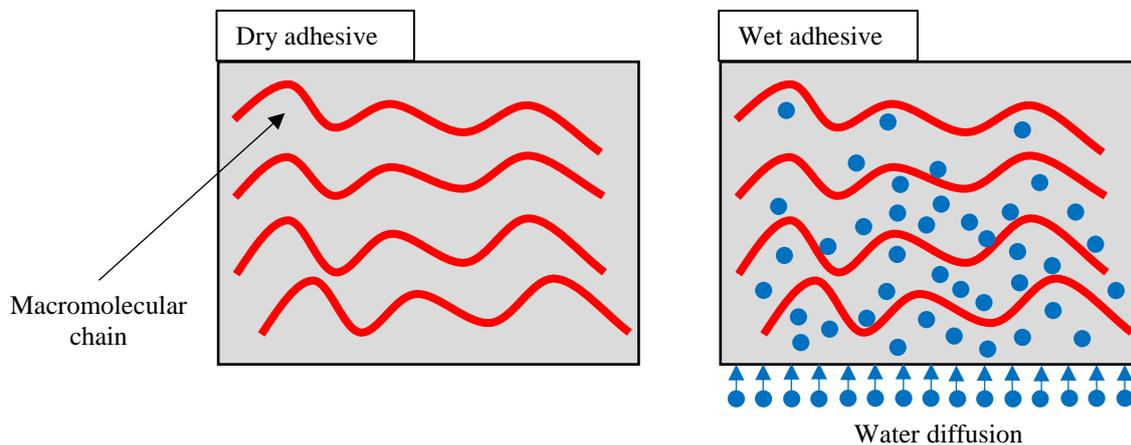
**Fig. 1.** Water diffusion in a polymer
