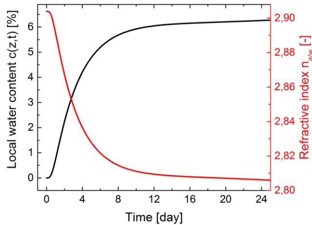
**Fig. 14.** Evolution of local water content and refractive index as a function of immersion time
