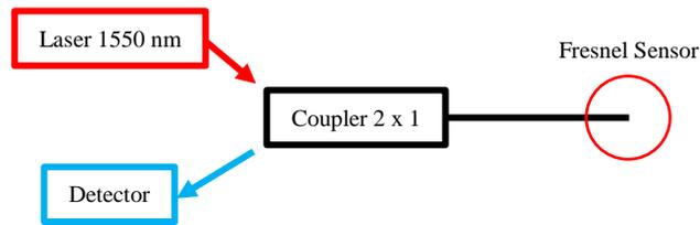
**Fig. 6.** Principle of measurement of Fresnel sensor
