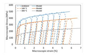
Fig. 3: Observed (dashed lines) and calculated (solid lines) macroscopic stress-strain curves at ambient, 100 and 300 °C
