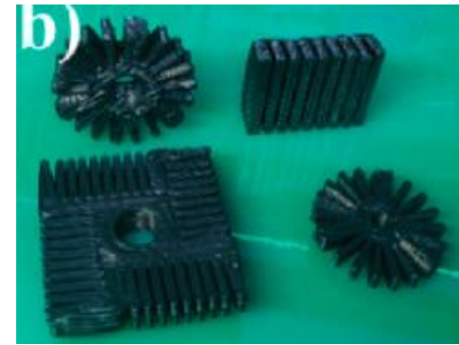
3D printed polymer filled with Graphene nanoplatelets 3
