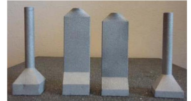
Aluminum 3D printed heat-pipe 3
