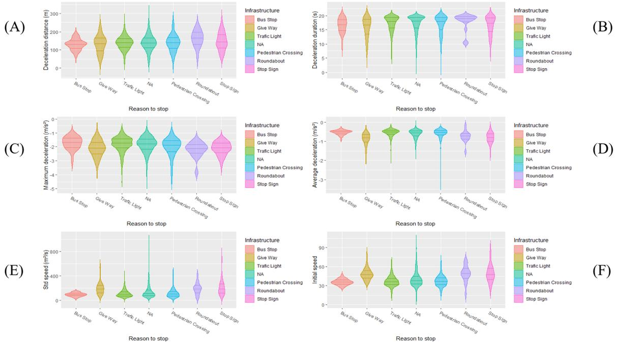
**Figure 2: Violins plots of the indicators according the reason for stopping: (A) Deceleration distance, (B) Deceleration duration, (C) Maximum deceleration, (D) Average deceleration, (E) Standard deviation of speed and (F) Initial speed.**
